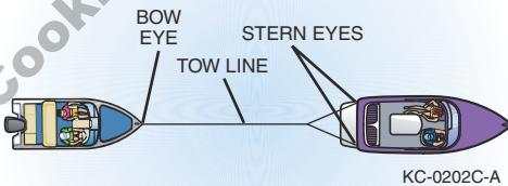
**WARNING** *Personal Injury Hazard: DO NOT attach tow lines to cleats, watersport line point, wake tower, or eyes used for docking; use only designated strong points. Death or serious injury could occur if lines and/or hardware fail while they are under extreme tension.*
