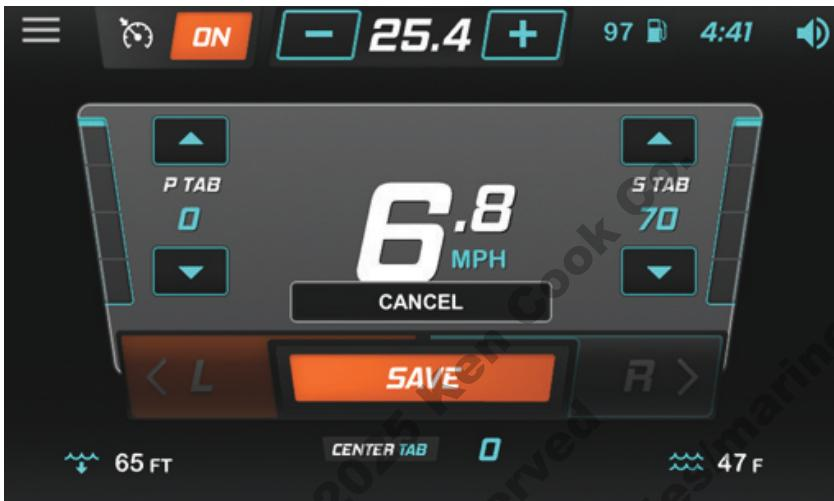
Fully adjust the Port and Starboard tabs via the “up” and “down” arrows.
