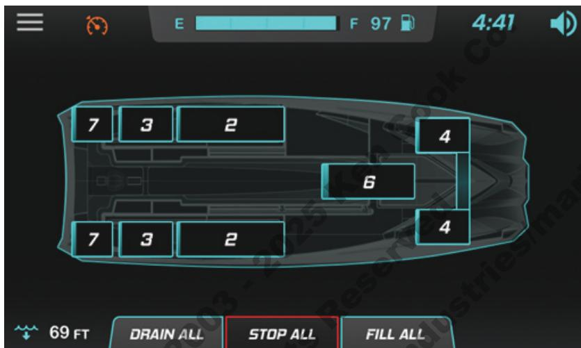
Individual ballasts may be filled or emptied. Touch the ballast, then touch “Fill” or “Drain.” Touch “Stop All” to halt the process.
